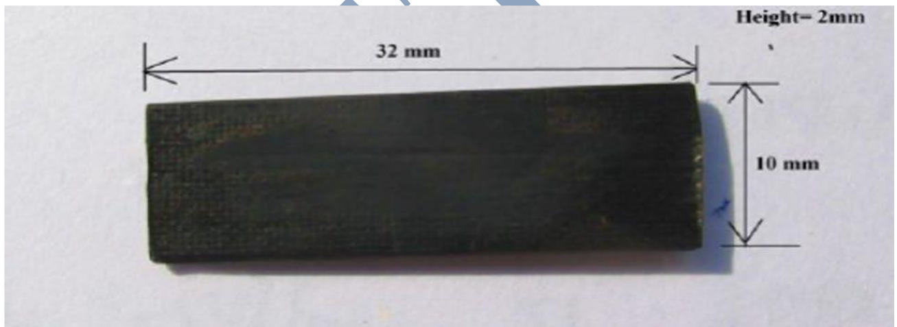
Fig. 1 CNT-reinforced 10-layered carbon fiber Nano composite
