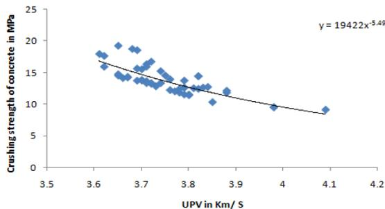
FIG. Relation between UPV and crushing strength:-
