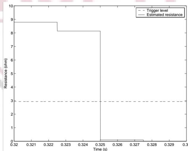
Figure 4: Estimated Resistance during a Fault
