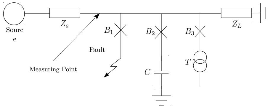
Figure 2: Single Line Diagram for Fault Analysis
