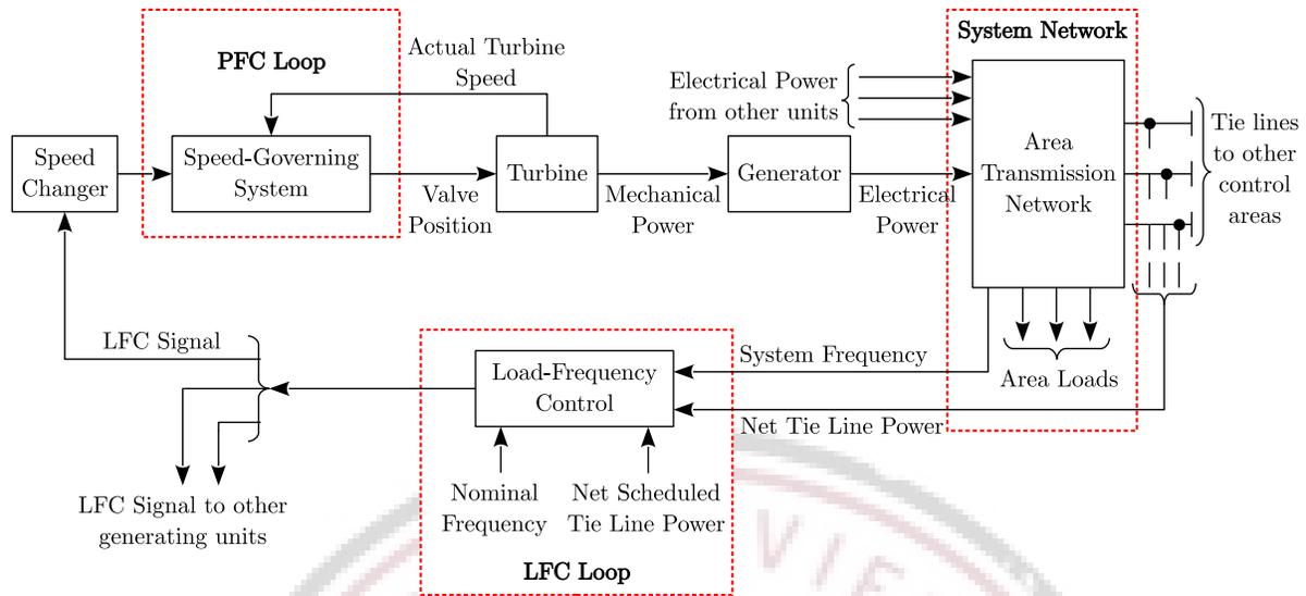
Figure 1: The Basic Schematic of Load-Frequency Control in Power System
