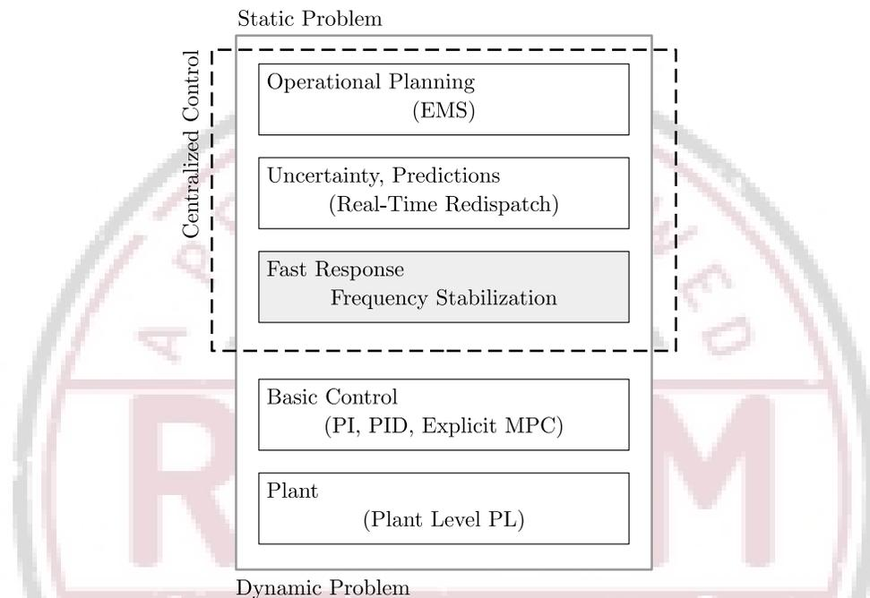
Figure 3: Hierarchy of Controllers in Centralized Control Scheme
