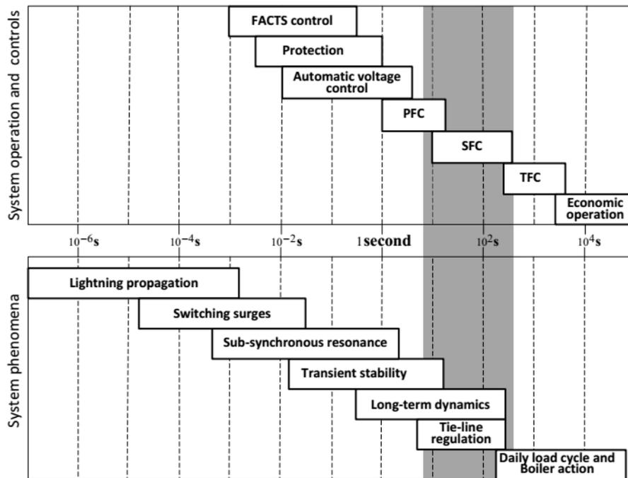
Figure 2: Time Scale of Dynamic Phenomena in Power System Control
