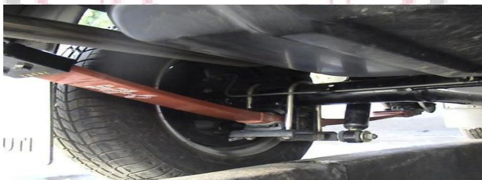
**Figure 1** New generation composite leaf springs
