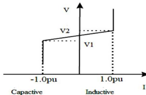
**Fig. 9 V-I characteristics of DSTACOM**
