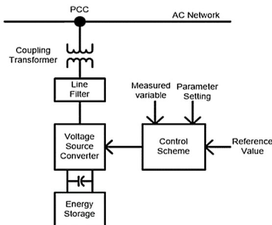
**Fig-3 shows the architecture of the D-STATCOM.**
