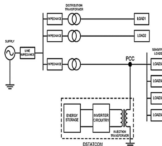
**Fig. 4 shows the connection of the D-STATCOM with the transmission line or distribution network.**
