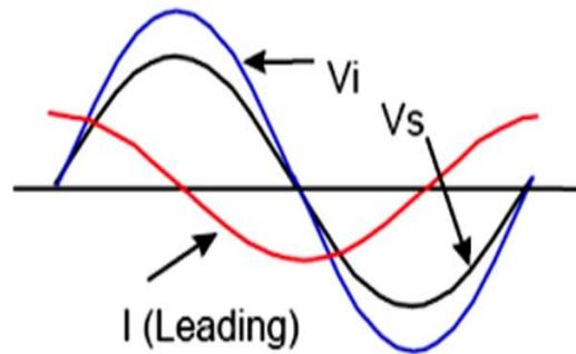
**Fig. 7 Capacitive operation**
