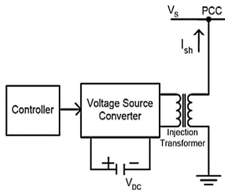
**Fig. 5 single line schematic of a D-STATCOM converter**
