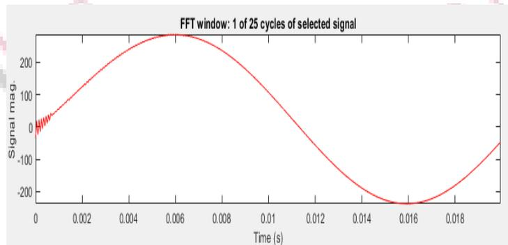
Figure 8 FFT analysis of Current at the loading line in system 1 with loads from area-1
