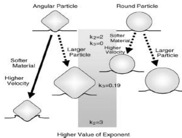
Fig. 4 Model of the effects of impact parameters
