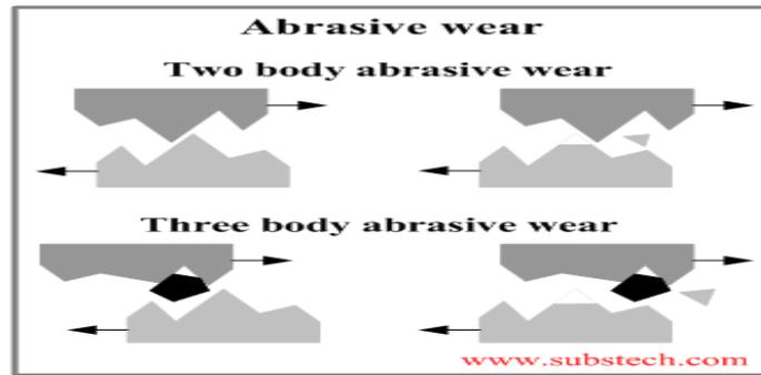
**Fig.2** Schematic representations of the abrasion wear mechanism.
