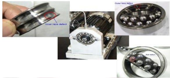
Figure 5 The Motor Bearing Fault
