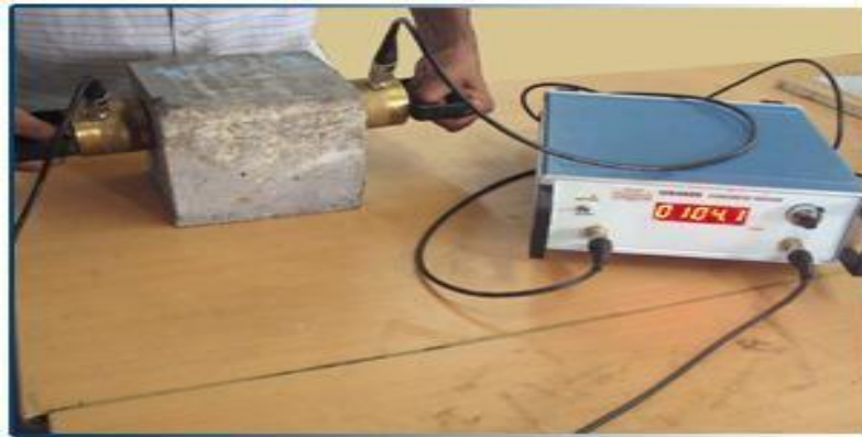
Figure 9 Ultrasonic Pulse Velocity
