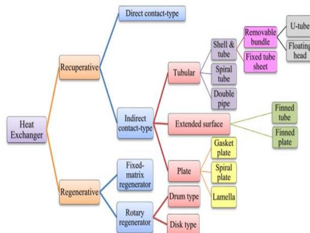
Figure 10 Classification of heat exchangers
