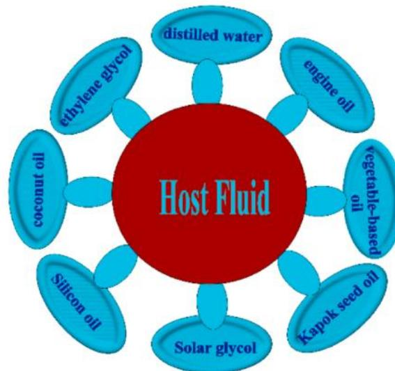
Figure 3 Some base fluids used as host medium of dispersed nanoparticles [5]
