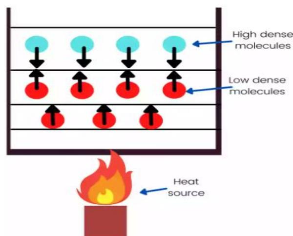
Figure 6 Free Convective Heat Transfer
