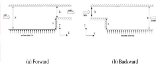
Figure 1 Facing Step Channel [1]
