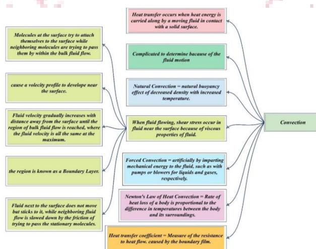
Figure 7 Types of heat transfer mechanisms and their subdivisions [10]
