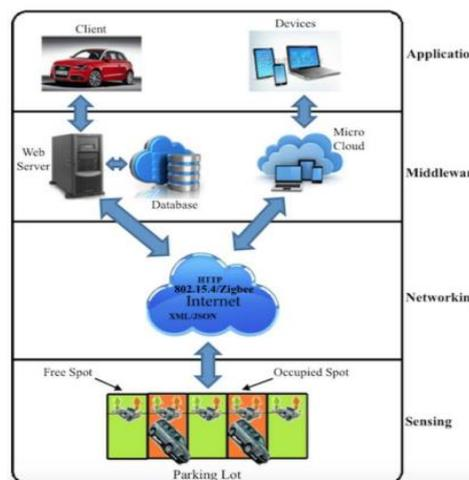
Figure 1 Smart parking system architecture [4]
