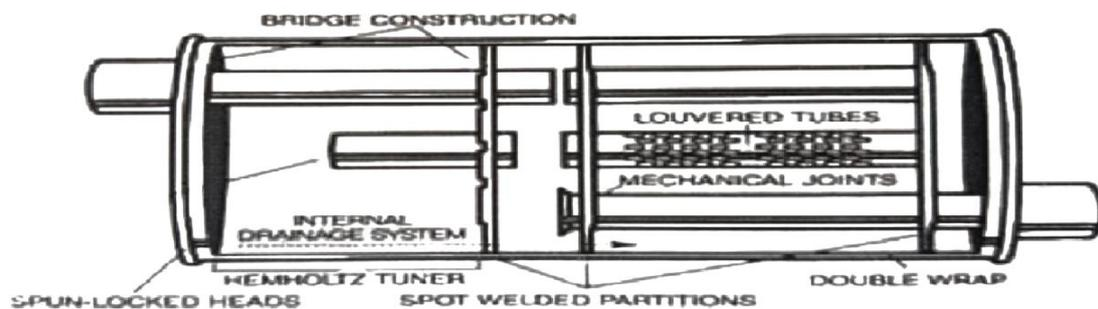
Figure 2 Sectional view of the muffler
