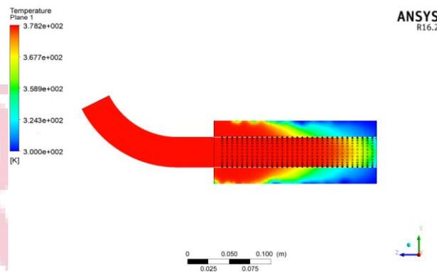
**Figure 11 Temperature contour for case 2**
