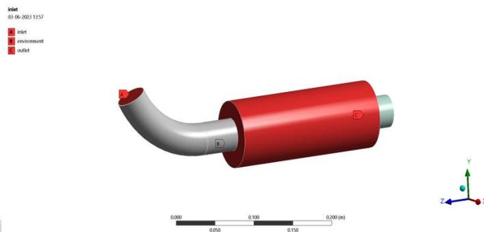
**Figure3 Boundary condition applied**
