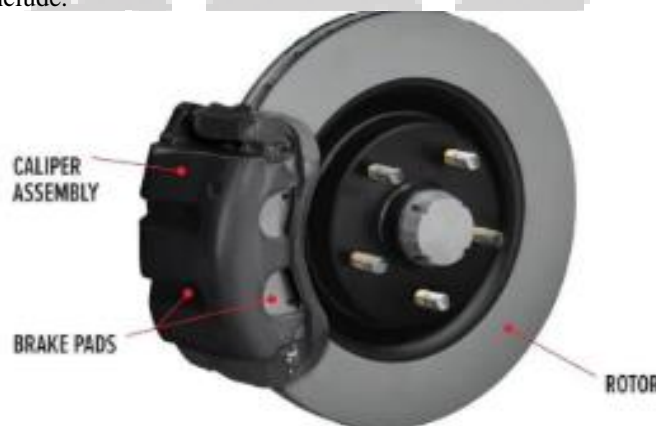
Fig. 3 – Rotors and brake pad assembly
