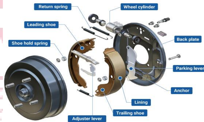
Fig. 1.3 Drum brakes consist of a brake drum
